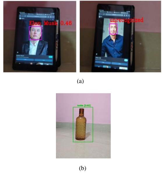
Fig. 6. View of Leo through head-mounted camera for (a) face detection and recognition (b) object detection
